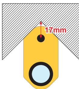
This is good for surveying on the corner of 90 degree.
