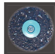
Bright field of view (optical plummet)
