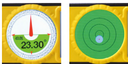
2 Measuring modes Circular level & Angle measure
