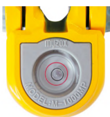
Circular level (40° / 2mm)
