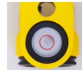
Circular level (40° / 2mm)
