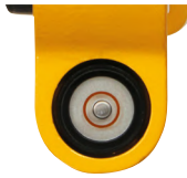
Circular level (30' / 2mm)
