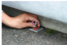
Circular level PC-40L (46° / 2mm)
