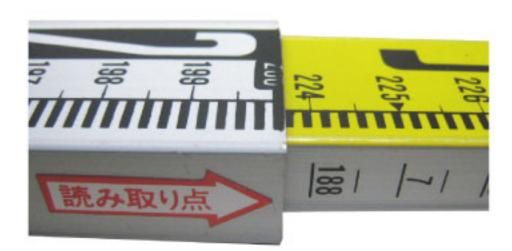
Reading point on hand help to check easily.
