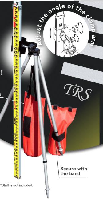
\*Do not use the product with the staff extended beyond 3m. \*Ensure the surrounding area is safe and use the product on stable ground. \*Tighten all the clamp arm screws securely before use.
