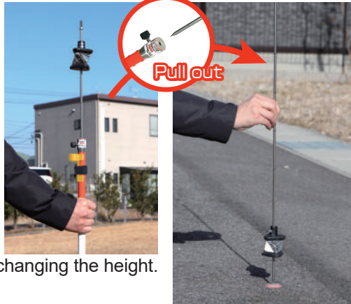
Use the inner pin pole alone for precision measurement.
