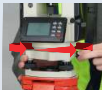
Shifting-type tribrach (35mm screw type only)
