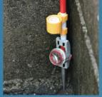
0.7inch compact prism M-700CP2 is the best for narrow places; by the wall and at the corner. Add 4.5mm when measuring by the wall.
