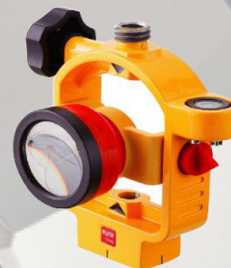
1.5 inch Prism 0mm / 30mm offset
